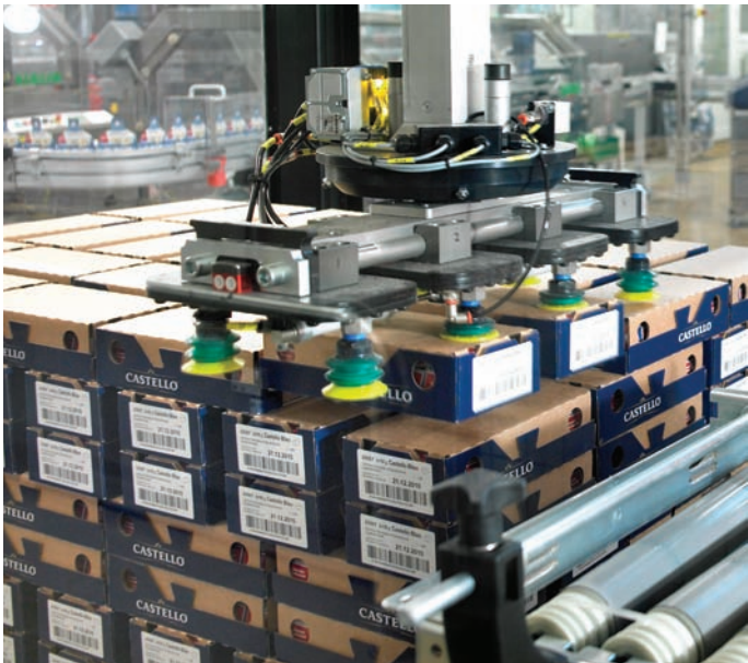
The special multifunctional gripper collects up to 4 cartons at a time and places them on the pallet with spacing to ensure correct cooling during storage.
